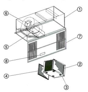
MOUNTING: Installs in a T-bar drop ceiling, replacing one 2' x 4' tile. CFM RATING: Variable between 930-1,020 CFM (1,575-1,750 m<sup>3</sup>/h) (high speed) and 350-875 CFM (600-1,500 m3/h) (low speed). The motor/ blower combination is capable of providing 1,800 CFM (3,050 m<sup>3</sup>/h) in free air. ELECTRICAL: 115 volts/60 Hz or 230 v/50 Hz @ 6.4 amps, 740 watts maximum WEIGHT: 130 lbs.-shipping, (59 kg)
